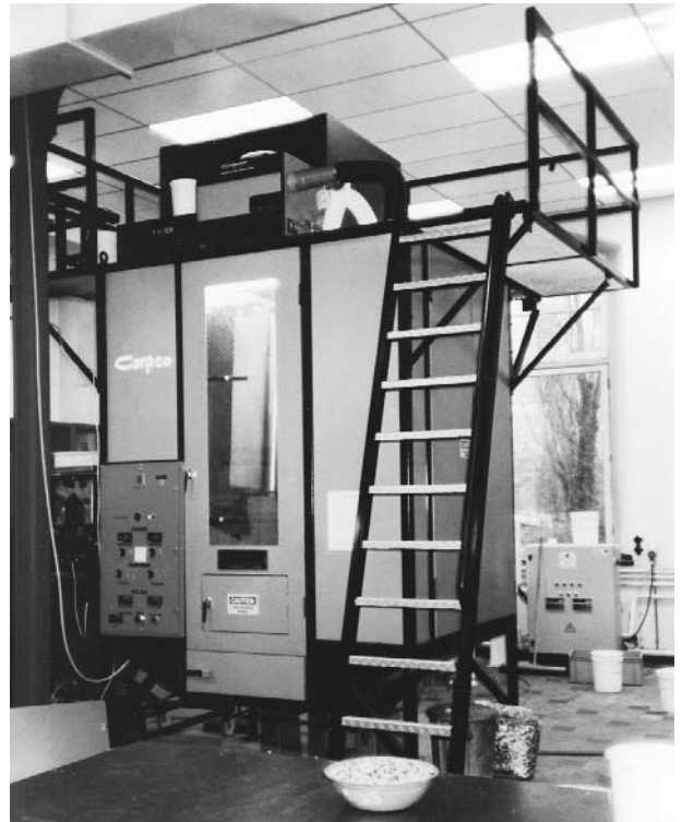
FIG. 19-62 New Triboelectric separator for separation of PVC from other plastics. (Courtesy Carpro, Inc.)
