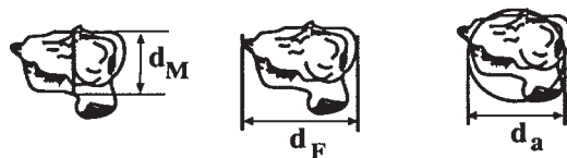
FIG. 20-5 Statistical (Martin's and Feret's) and projected area diameters for an irregular particle.
