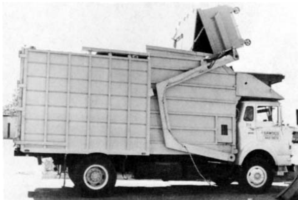
FIG. 25-61 Typical front-loading compactor used in a stationary-container collection system.
