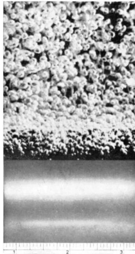
FIG. 14-95a Comparison of bubbles from a porous septum and from a perforated-pipe sparger. Air in water at 70°F. Grade 25 porous-carbon diffuser operated under a pressure differential of 13.7 in of water.
